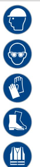
The head protection serves to protect against falling and flying parts and materials. It also protects the head from bumping into hard objects.
