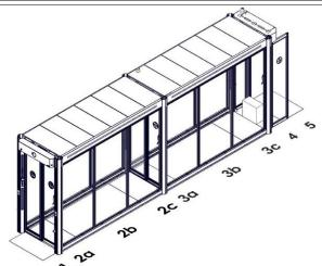
A person or object remains under the exit door or in zone 4, the exit door opens.
