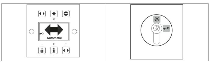
If the "Locked" operating mode is present, it must be protected, for example, by means of an access code or a key in such a way that only authorized personnel can set a different operating mode.
