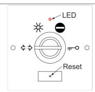
The BDE-M mechanical operating unit is equipped with a key switch. This key switch can be used to set the various operating modes. The key switch can be removed in any position.
